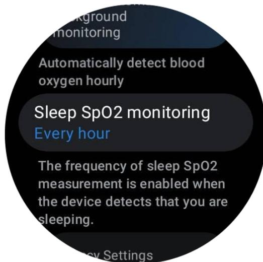
2. Sleep blood oxygen monitoring frequency can be set to one of three modes: once every hour, once every 30 minutes, or real-time monitoring. Sleep blood oxygen data will be displayed according to the chosen monitoring frequency.
