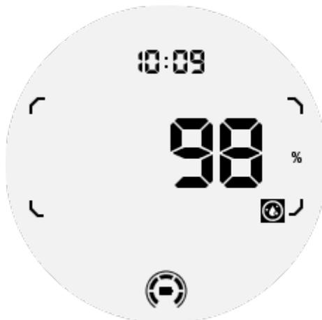
To ensure accurate measurement, please avoid loose wearing, excessive tilting or shaking during blood oxygen detection. If any of these conditions occur, the device will prompt "FAIL".
