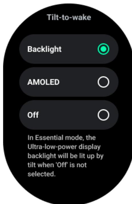
In general, there are two methods to activate the backlight: raising your wrist or rotating the crown more than 180 degrees. The backlight will automatically turn off after a timeout or when you lower your wrist. Additionally, the ULP display will be locked to prevent accidental operations.
