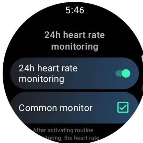
1. Common monitoring: Data is displayed at a frequency of one data point every 10 minutes.
